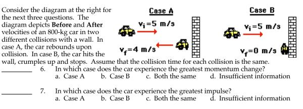
8. The impulse encountered by the 800-kg car in case A has a magnitude of \_\_\_\_\_ N•s.
